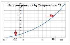
put from your heater. The pressure in a propane tank at -20°F drops by a factor of 10 times from that at 80°F (from 123 PSI to 12 PSI).
